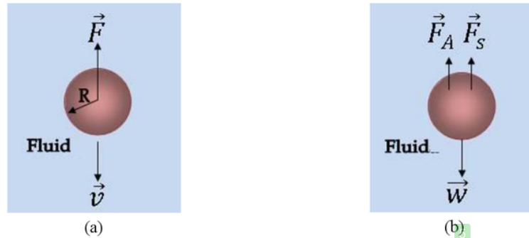
Figure 1 (a) The ball which is moving in a fluid always gets a friction force in the opposite direction of the motion of the object, (b) The force which is acting on the ball when falls into the fluid. (adaptation from [5])
